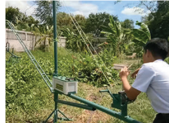
Semi-automatic system water hyacinth collecting machine
