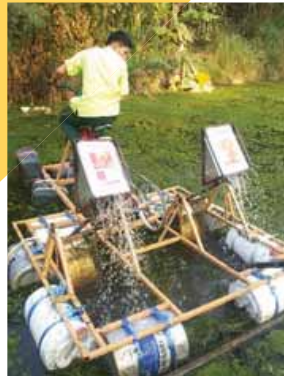
Human-power water turbine to add more oxygen into the canal
