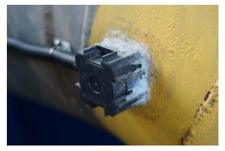
Fig1. Vibration and Temperature Sensor
