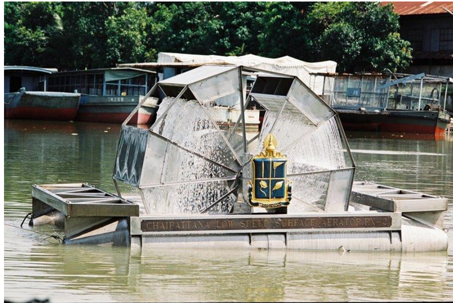
Low speed surface Aerator
